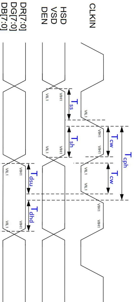
Figure : Input signal timing
